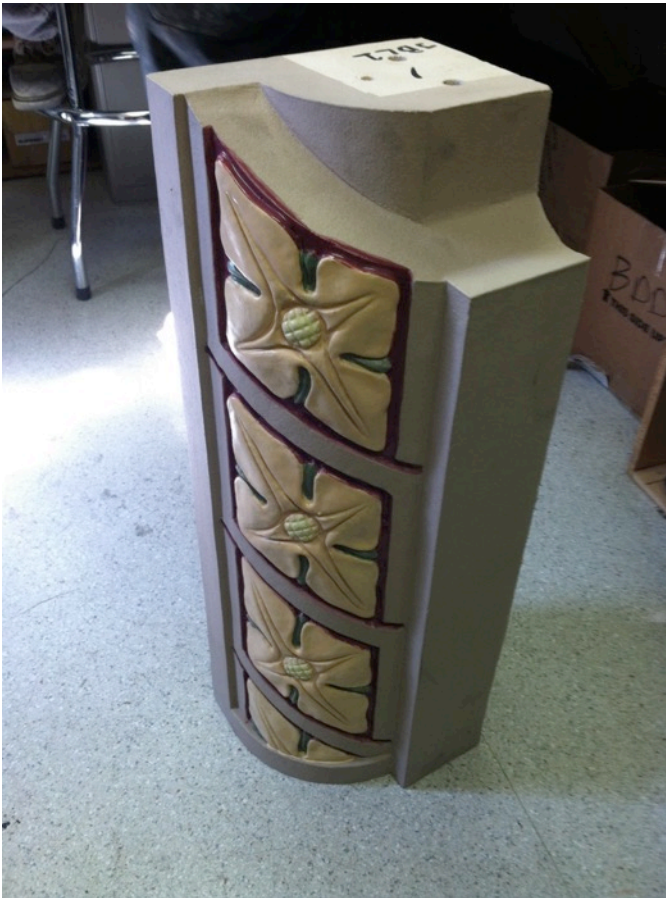
Fig. 5.64: Replicated T.-C. Window Surround
