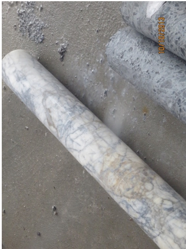
Fig. 5.21: Removed Marble Column Cores
