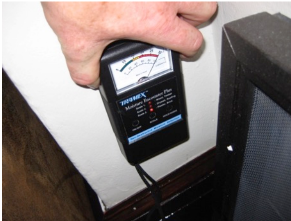
Fig. 3.74: High Moisture Below Sill
