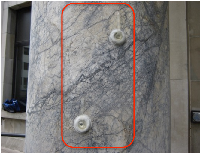
Fig. 2.23: RILEM Absorption Testing of Col.
